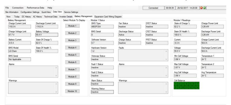
Charge Current Limit: The maximum charge current allowed at the time
