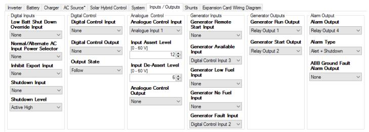
Low Batt Shutdown Override Input function is also known as the "Just Go" control. In case of emergency, even if the batteries would normally be considered too flat to safely run the inverter, activating this input will force the inverter to run, until there is insufficient battery power left to maintain the load. This is considered essential if, say, phones or a fire pump MUST be operated.
