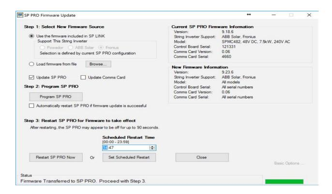
Step 3 If Automatically restart SP PRO if firmware update is successful was not checked then the SP PRO must be restart at this stage to complete the firmware update.
