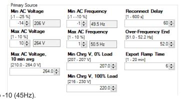
Max AC Voltage, 10 min avg. This setting is only used in a Solar Hybrid system. For off grid systems set it to the maximum value of 264V. If the 10 minute average of AC Source Voltage goes above this value then the SP PRO will disconnect from the AC source. The default of 255V is suitable for Australia. Set this to 248V for New Zealand.
