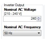
Nominal AC Frequency is set to 50Hz and cannot be changed when Powador Managed AC Coupled Solar is enabled. When ABB managed AC coupling or Fronius Managed AC coupling is enabled, then 50Hz or 60 Hz may be selected
