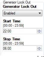
If the system design calls for very little, or infrequent generator input it is wise to run the generator periodically to keep the internal parts of the motor covered with oil and to keep the starting battery charged.
