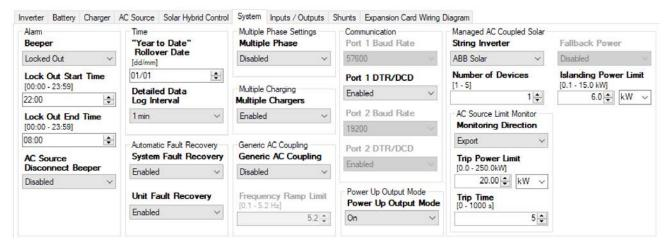
The SP PRO is configured to recognise, and report, a number of events that can cause damage to the system, such as overloads, low voltage batteries. These events can be announced by a beeper within the SP PRO.
