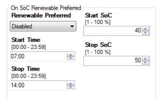
If the solar input does not meet the usual consumption level you can start the day with a compensating charge that will enable the normal solar input to fully charge the batteries.
