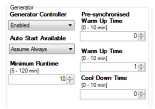
Minimum Runtime determines the shortest time the generator will run. This is to ensure the generator wont start and stop too frequently.
