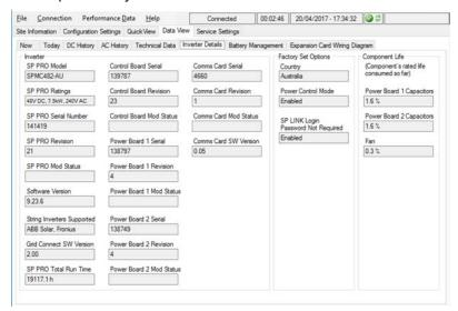
In the INVERTER section we show you the SOFTWARE VERSION and hardware that is currently installed in the inverter. From time to time, as Selectronic designs new features for the SP PRO, new revisions of software may become available from our web site. Generally, there is no need to update the SP PRO unless you need the new features made available.
