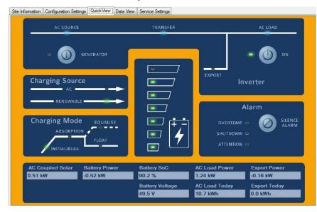
QuickView can easily be accessed directly from the computers desktop. Click the SP LINK Auto QuickView icon (installed automatically with SP LINK) and the last site will automatically be loaded and a connection (if possible) established.
