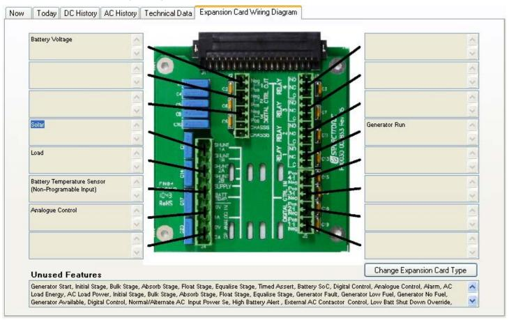
The Unused Features display lists all input and output functions that have not been allocated to an input or output.
