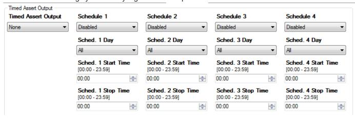
The final section controls the Solar Hybrid function allowing for a Backup Generator to be automatically controlled during times of Grid failure.
