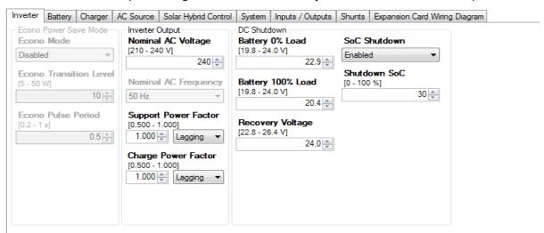
With **Econo Mode** disabled the inverter will run continuously regardless of the AC load. When Enabled, the SP PRO will go to "sleep" when the AC load power is below the Econo Transition Level for more than 30 seconds. It will "wake up" again and run the load once the AC load goes above the **Econo Transition level**.
