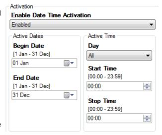
The digital input set in **Activation Input** is also used to activate the Priority schedule. This input will activate the Priority schedule regardless of the Date Time Activation. When set to "Rising" the Priority will be active when the input is high and inactive when the input is low. A "Falling" setting will control the priority in the opposite sense..
