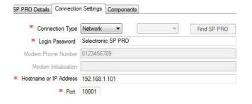
Connection to the SP LINK via a local NETWORK is made using the optional SP PRO Ethernet Adaptor Lead, stock code 005081. enter the HOSTNAME or IP ADDRESS of the serial/Ethernet adaptor and the IP PORT number of the serial connection to the SP PRO.
