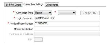
For Modem connections, select the PC COM port that the modem is connected to. Enter the MODEM PHONE NUMBER. This is the number that SP LINK will dial when you select Connect. Modem Initialisation can be left blank when using Selectronic supplied modems but may be required for other modem types.
