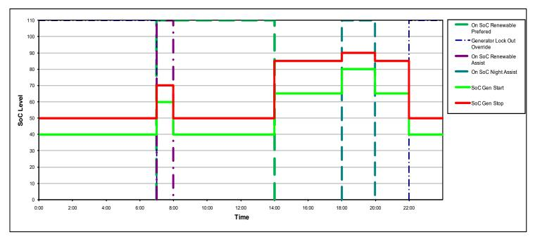
When you get up in the morning, before the solar panels are working at their best, the generator runs for an hour or so while you are cooking, or heating the bathroom for the kids, and starts the day with a support charge (see SoC Renewable Assist).
