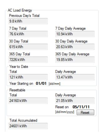
This is the total AC input contributed by the motor generator or by the mains grid.
