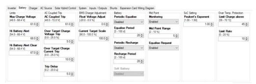
Max Voltage Limit is the absolute maximum voltage produced by the charging section of the inverter in any charge stage.
