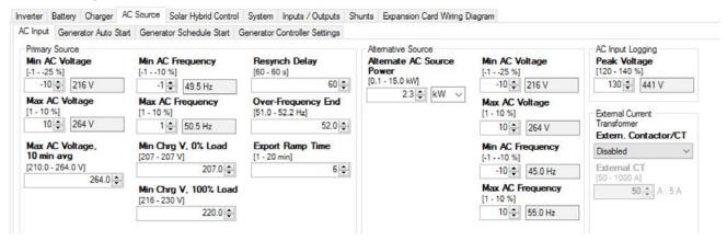
THE PRIMARY SOURCE configurations set the AC voltage and frequency at which the AC source will disconnect, when an export power limit occurs or when the charge power taken from the AC Source is limited.
