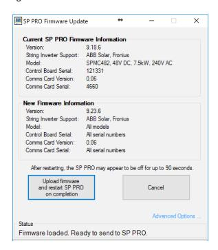
Once SP LINK connects to the SP PRO, the SP PRO Firmware Update window will appear. Select "Update Firmware and Restart SP PRO on Completion". If this option is disabled then the firmware is up to date.
