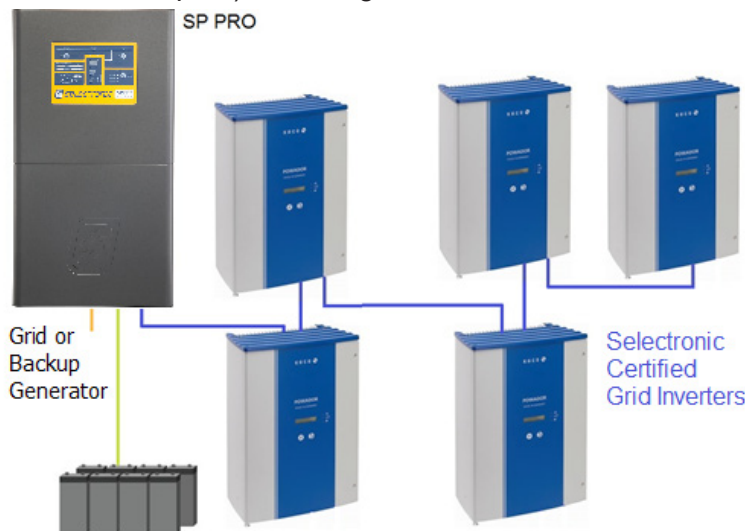
RS485 wired communications links between SP PRO and Selectronic Certified inverters
